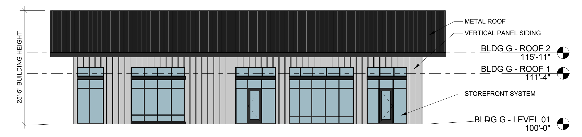
3 BUILDING G - NORTH ELEVATION 3/32" = 1'-0"
