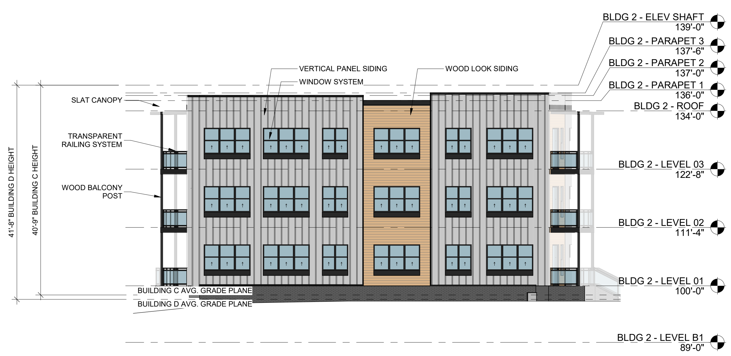
BUILDING C ELEVATION (BUILDING D MIRRORED) 6 3/32" = 1'-0"
