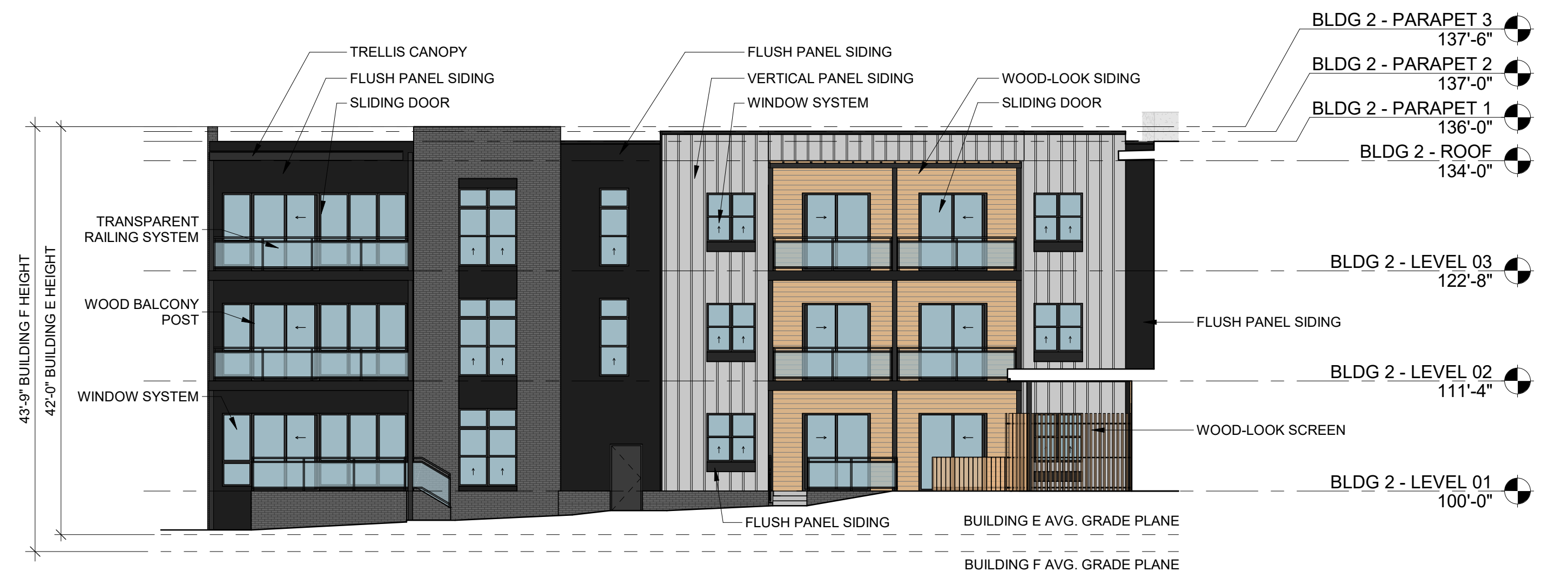
2 BUILDING E/F ELEVATION 3/32" = 1'-0"
