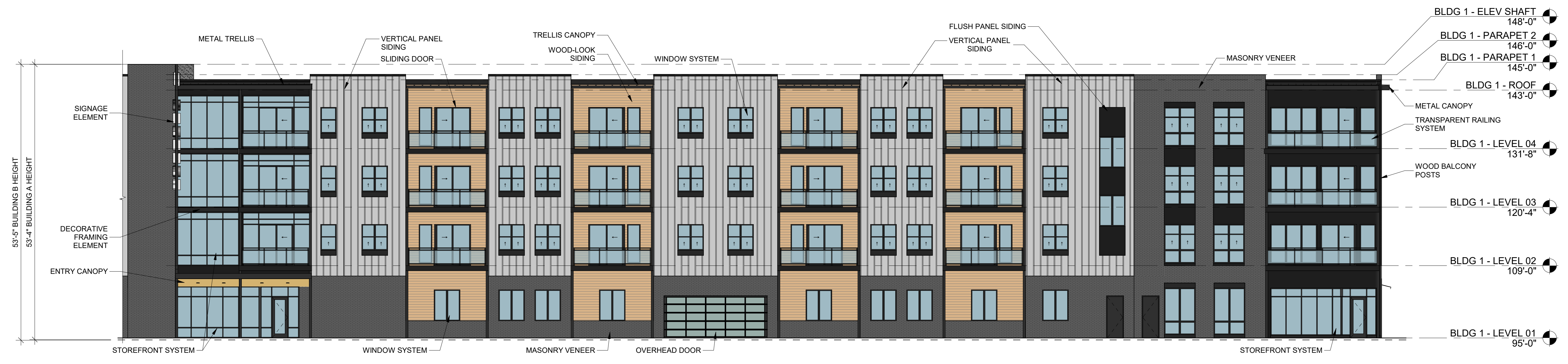
1 BUILDING A/B ELEVATION 3/32" = 1'-0"
