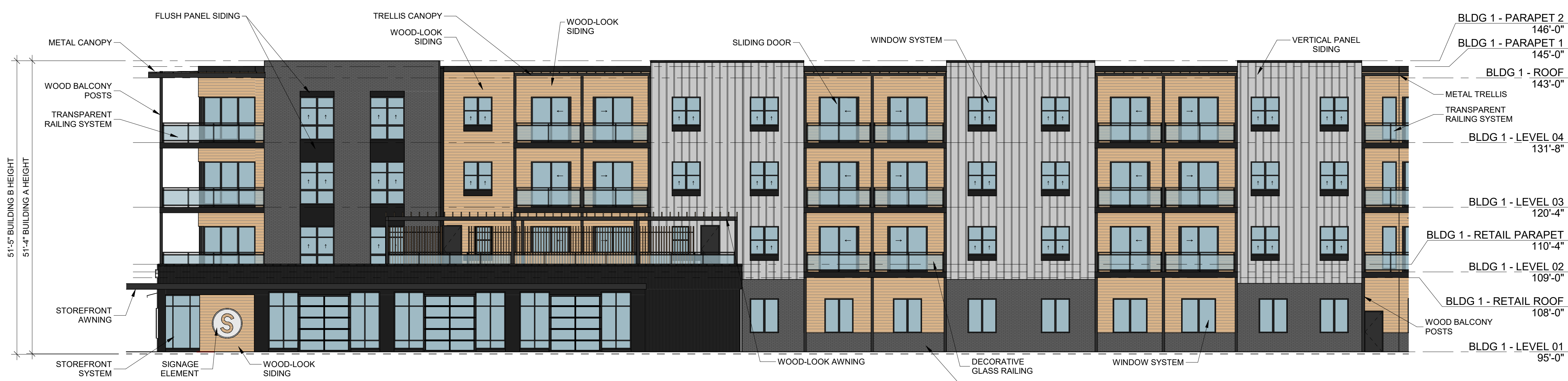
6 BUILDING A - SOUTH ELEVATION 3/32" = 1'-0"
