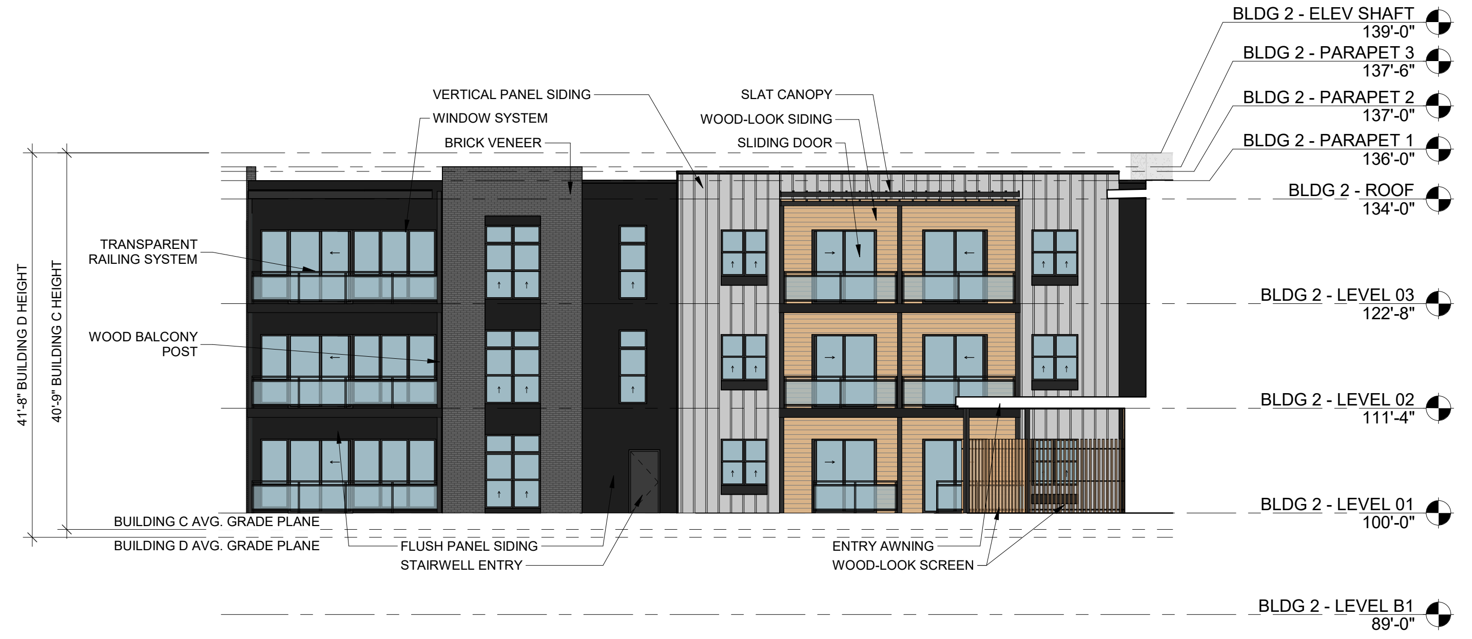
BUILDING C ELEVATION (BUILDING D MIRRORED) 5 3/32" = 1'-0"
